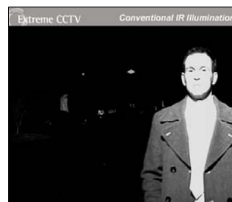
Conventional Infrared Illumination Background under-exposed. Foreground over-exposed.
