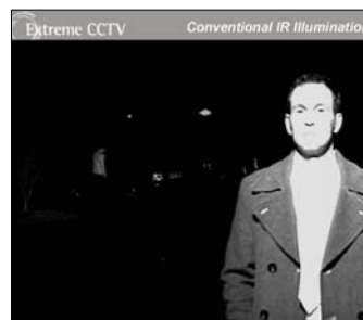
Conventional IR Illumination Background under-exposed. Foreground over-exposed.
