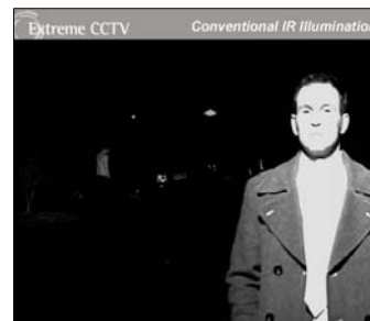
Conventional IR Illumination Background under-exposed. Foreground over-exposed.
