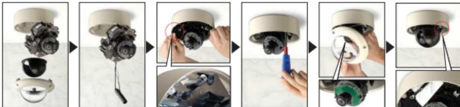
**1.** Pull out the camera unit by loosening the screws.\*1
