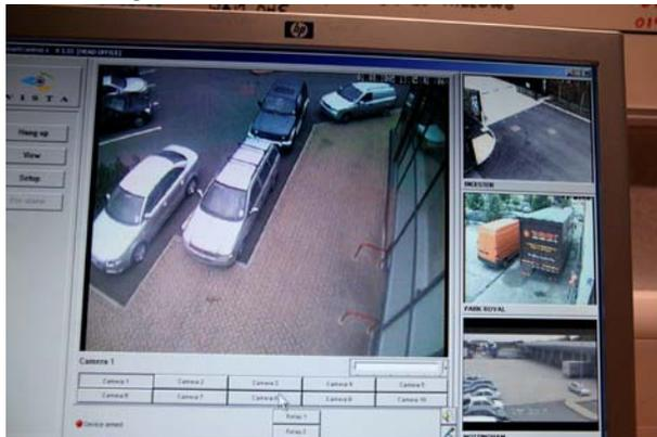
A rolling CCTV installation programme began once Vista SmartTel was identified as the standard transmission unit. UIS and Target have together identified a package of equipment, supplied by Norbain, for installation in all depots. Bosch cameras are used, with both static models (LTC 0455) and colour/monochrome domes (ENVD230). Other equipment in the depots includes monitors and digital
